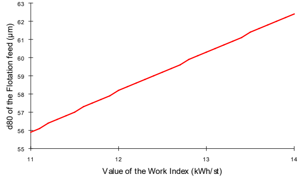
Figure 6 Evolution of the d80 of the Flotation feed versus the value of the Work Index
